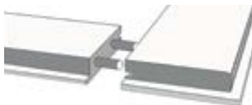
FRAMED CONSTRUCTION - structural elements connected with mounting pins
